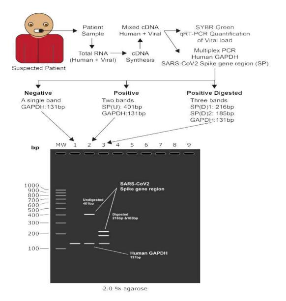
**Figure 2:** Simulated 2.0% agarose gel electrophoresis, MW: 100bp ladder; Lane 1 : Digested PCR amplicon from virus negative sample; Lane 2 : Undigested PCR amplicon; Lane 3 : Swa1 digested PCR amplicon.
